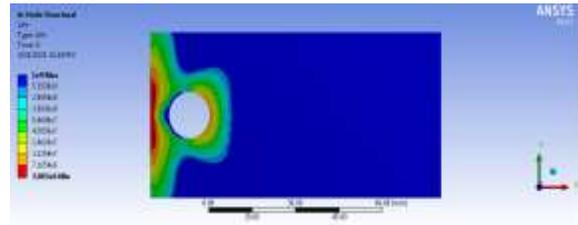
According to the plot, the maximum life at fastener hole and minimum at end of the specimen.
